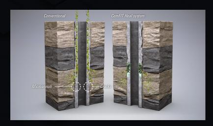
Conventional cement barriers (left) can develop cracks and microannuli caused by pressure changes and other stresses, allowing fluids to flow between zones and rise to the surface. The CemFIT Heal system (right) responds to any contact with oil or gas by automatically repairing and sealing itself.
