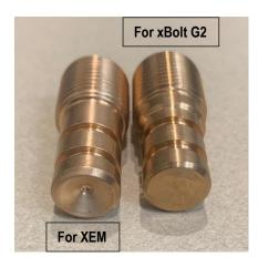
This new port plug still requires being installed using 42 ft/lbs of torque with blue 246 Loctite applied to the threads and the snap ring installed as a standard XEM application would.
