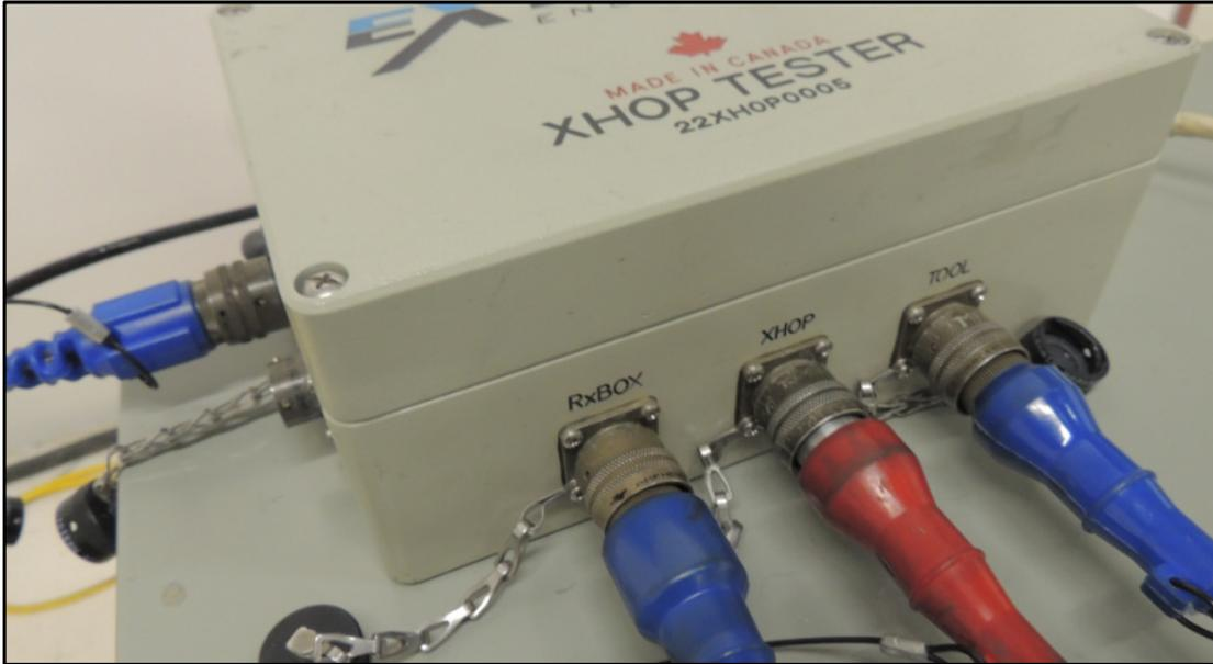
**Figure 24 Tool Port on XHop tester connected**
