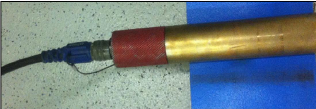
**Figure 25 Female ROTC attached to the bottom of the XEM**
