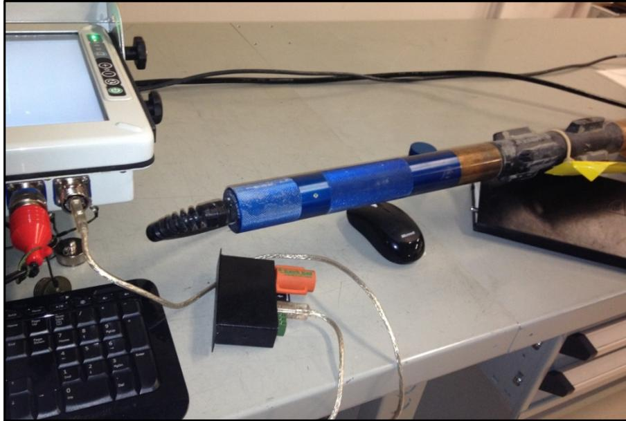
Figure 13 Male ROTC Connected to the XHop probe
