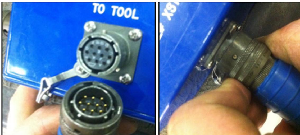
Figure 44 22CABL0016 connected to the system tester
