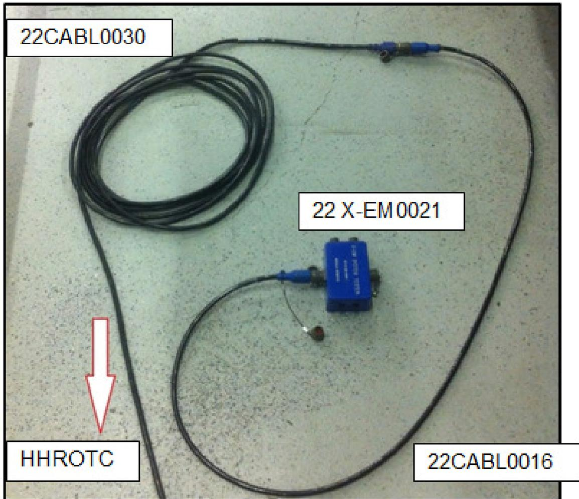
Figure 45 Hardware setup for programming the tool (In progress)
