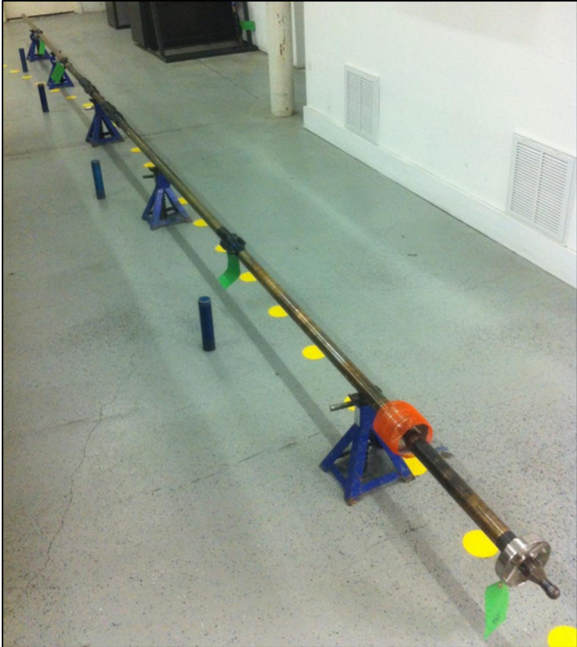
**Figure 25 XEM Tool String with DPG, XTX, Battery, DynamX, XGM**
