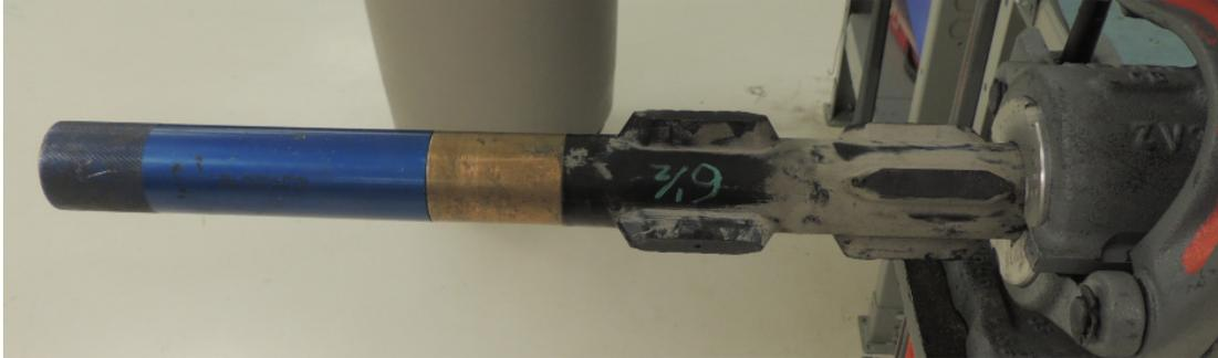
**Figure 5 Probe centralizer**
