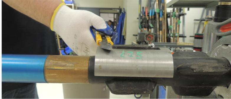
**Figure 9 shaving the rubber of the centralizer fin**
