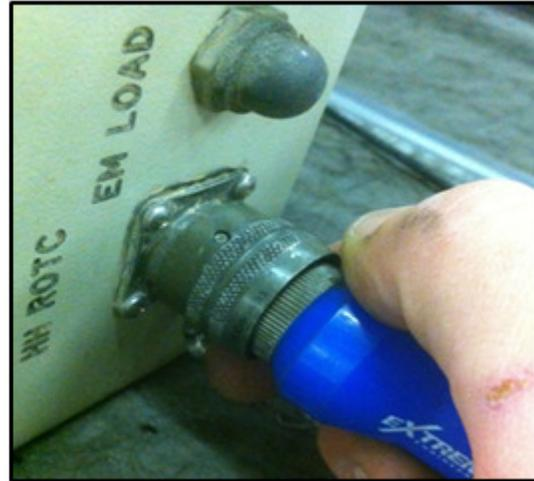
**Figure 48** 22CABL0016 connected to the “HH ROTC” port on the XTR
