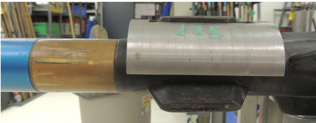
**Figure 8 Cutting jig placed on the top centralizer fin**
