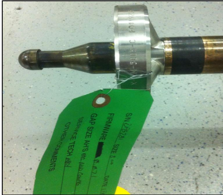
Figure 33 Green tag attached to probe
