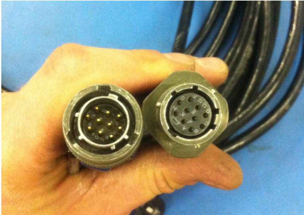
**Figure 38 ROTC extension Cable 22CABL0030 Male/ female connectors**
