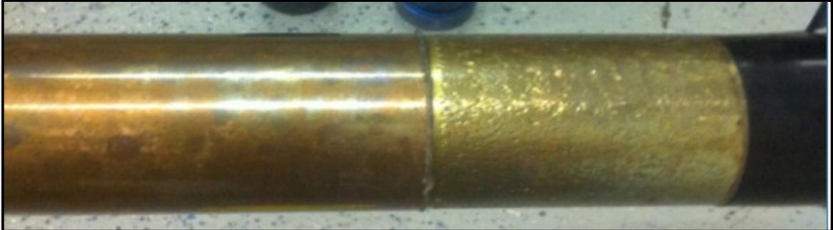
**Figure 20 DPG XTX Connection made up and torqued**
