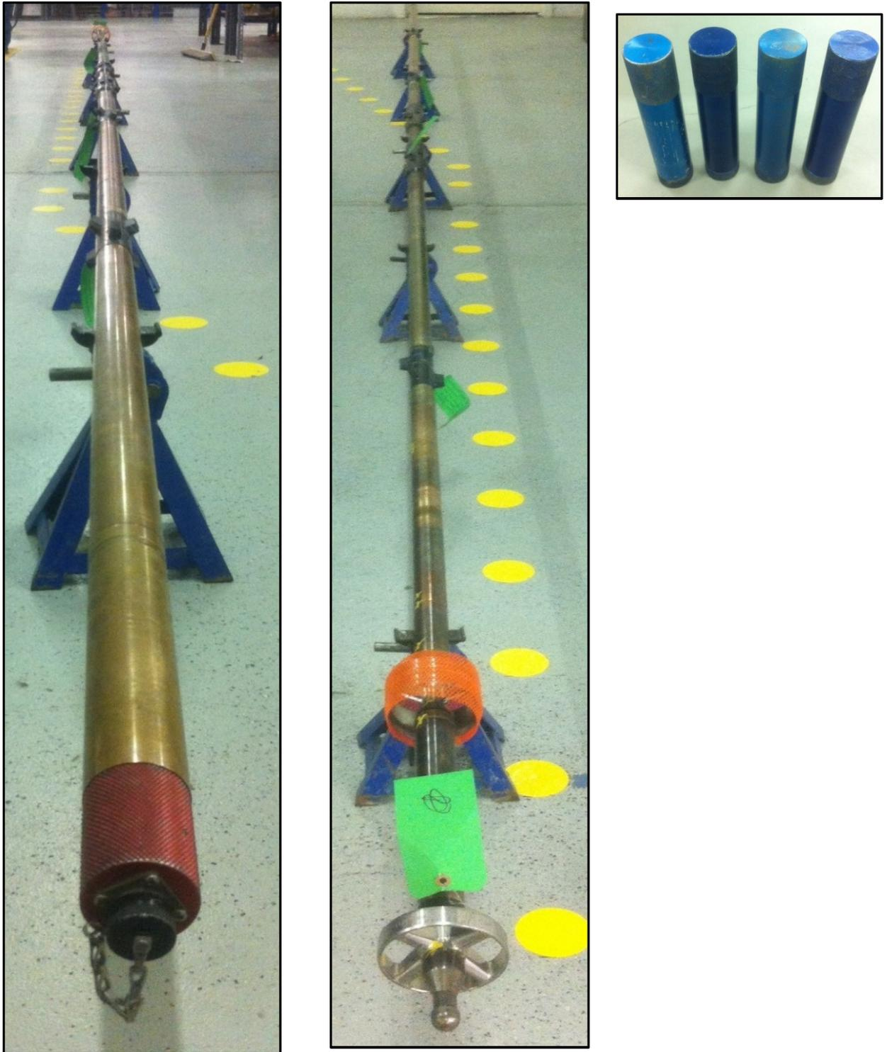
**Figure 28 Tool with female HHROT connection**
