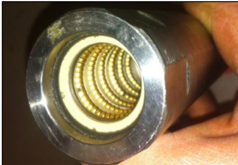
Figure 14 XTX female connector
