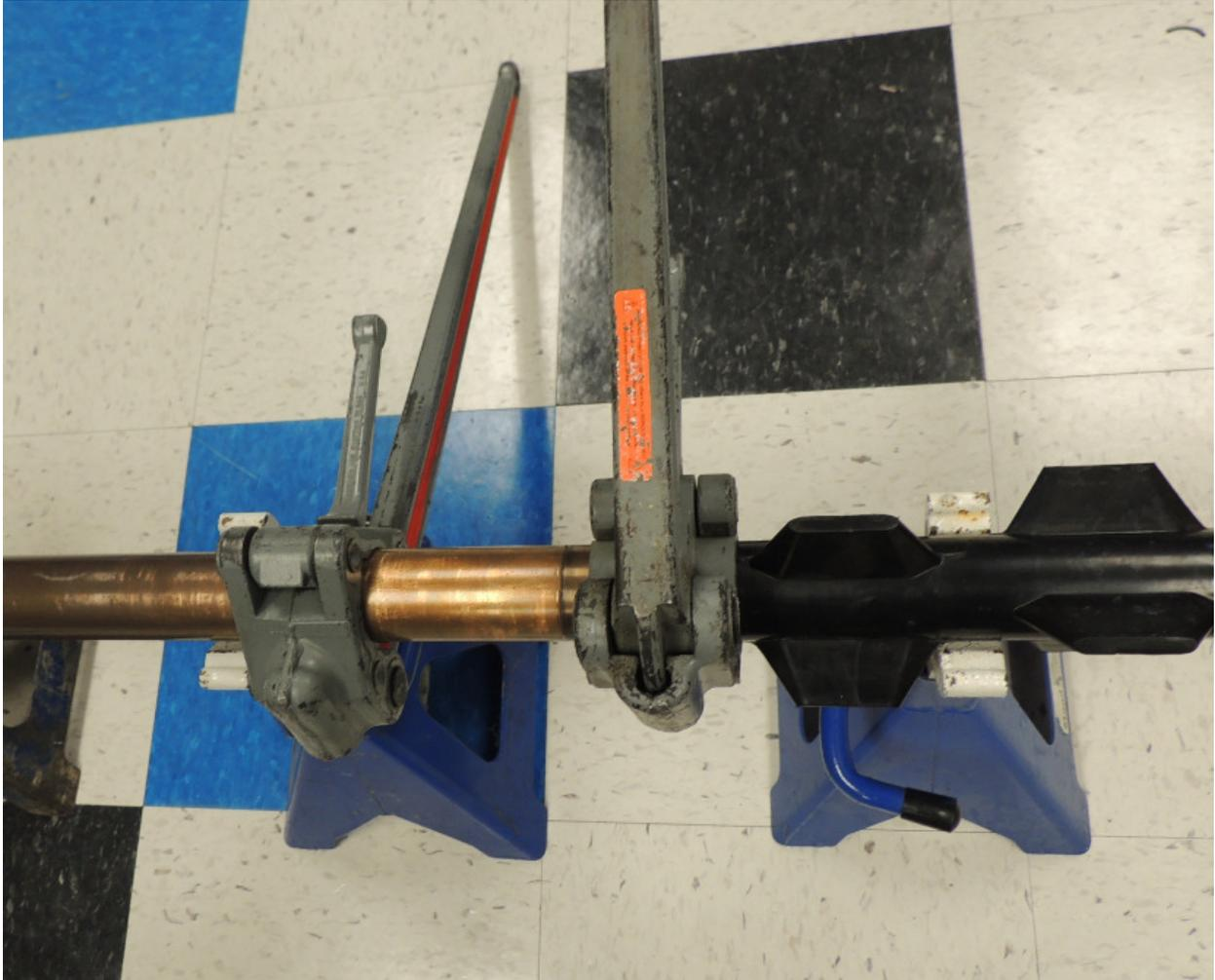
**Figure 19 XTX & DPG – Torque applied on connection**
