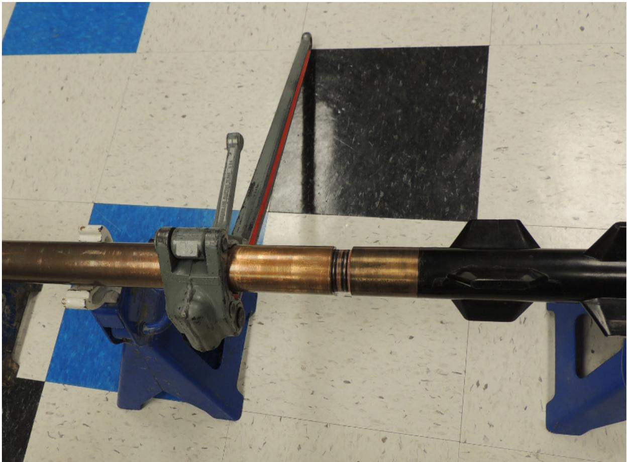
**Figure 16 Barrel wrench on DPG**
