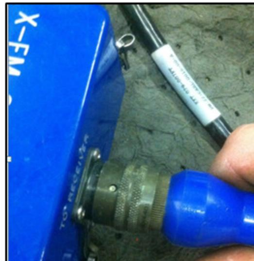
**Figure 49** 22CABL0016 connected to the “TO RECEIVER” port on the tester
