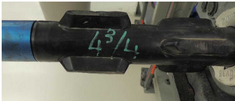
**Figure 11 Rubber removed from all centralizer fins**
