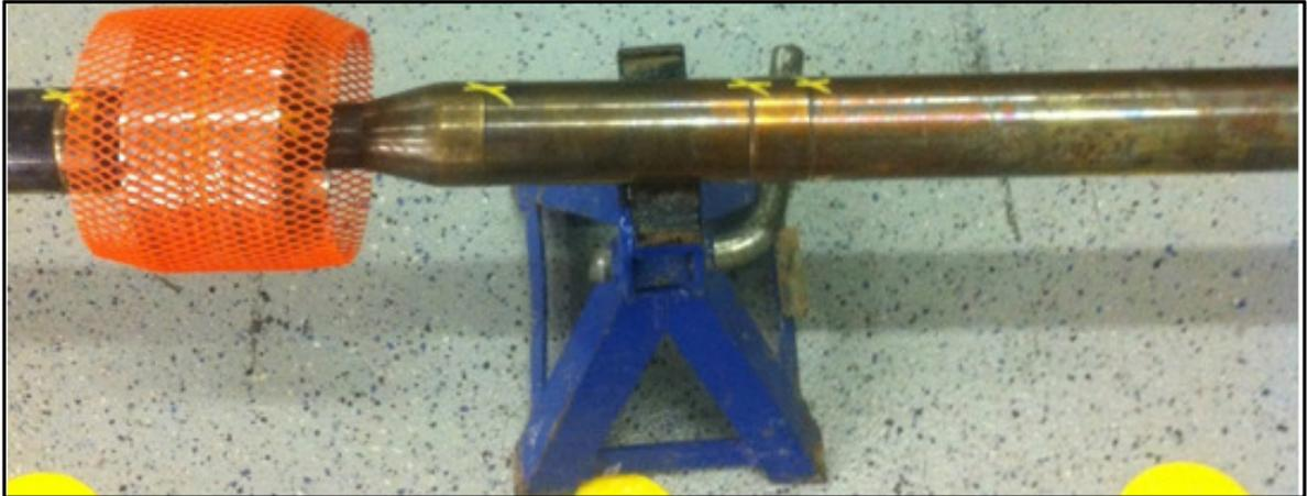
**Figure 31** Tool electrically connected to the ground through the jack stand
