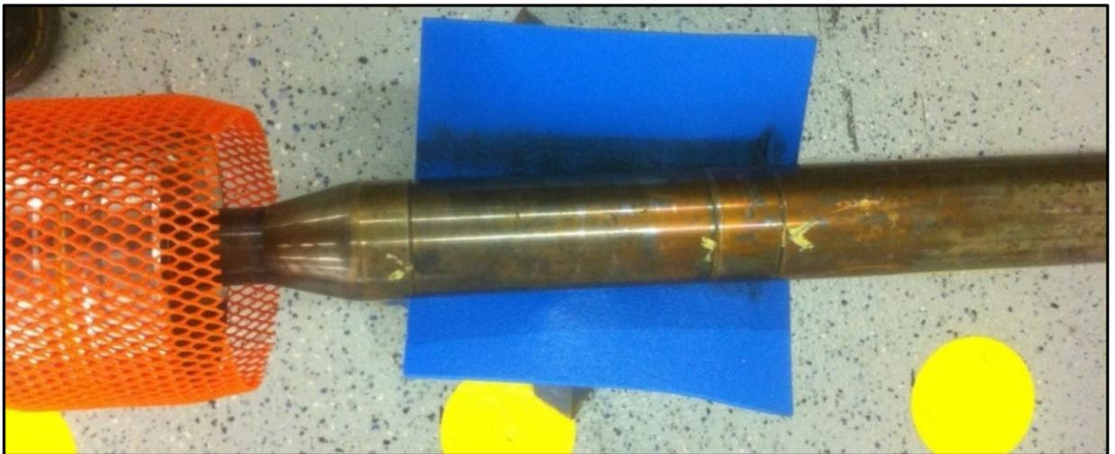
**Figure 32** Probe electrically isolated from the jack stand and ground
