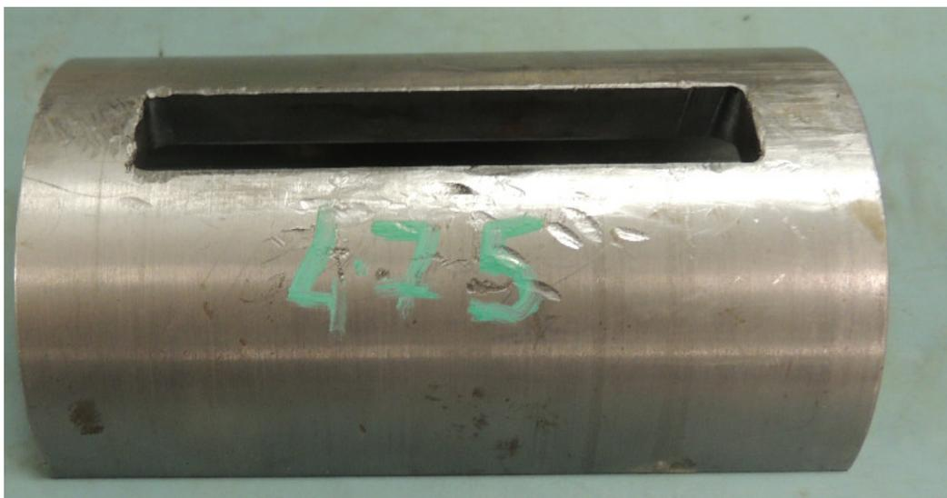
**Figure 6 centralizer cutting jig**
