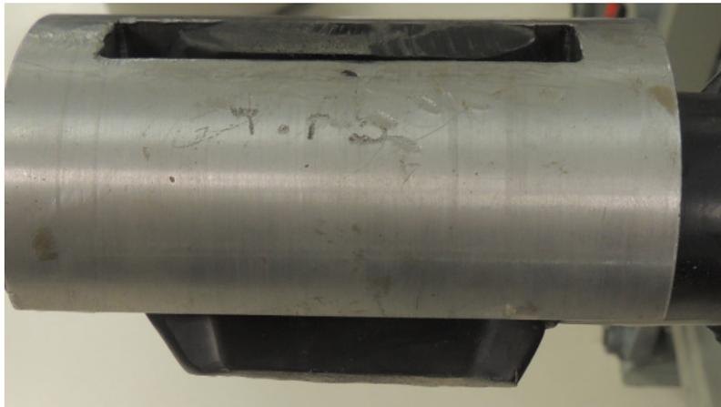
**Figure 10 Rubber removed from 1 x centralizer fin**
