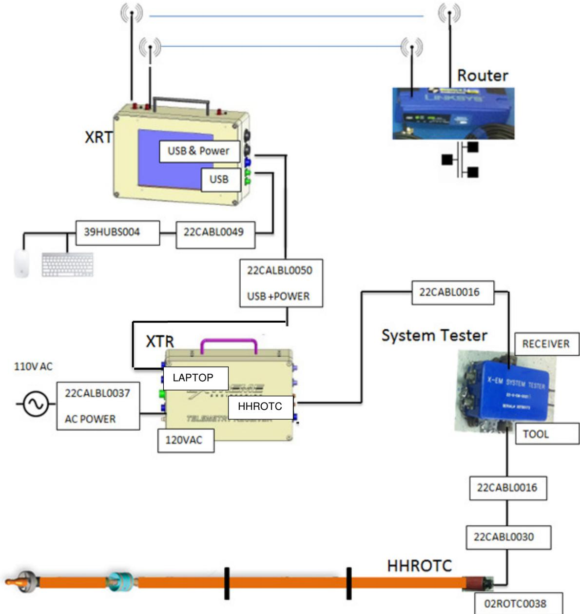
**Figure 36 Hardware setup for programming the tool**
