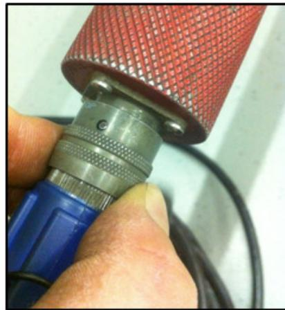
**Figure 39 22CABL0030 connected to the HHROTC**
