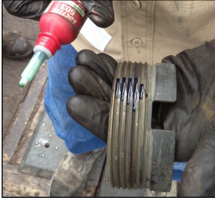
Figure 33 Loctite on Castle Ring
