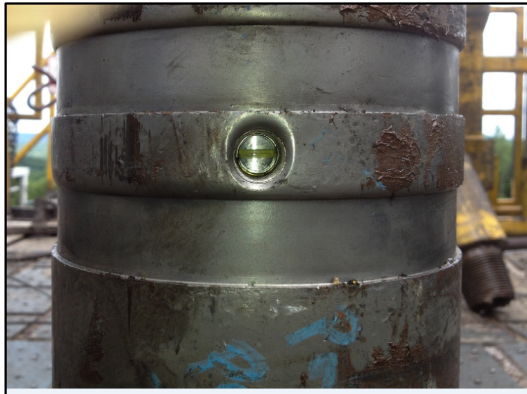
Figure 31 Yellow Paint/ Annular pressure channel visible on the Grounding spider
