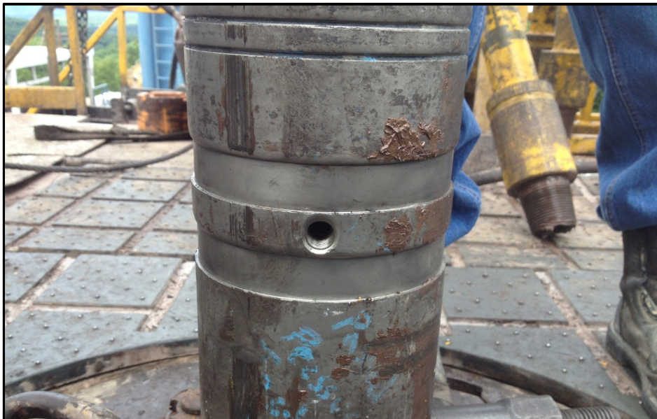
Figure 24 Grounding Set screw removed
