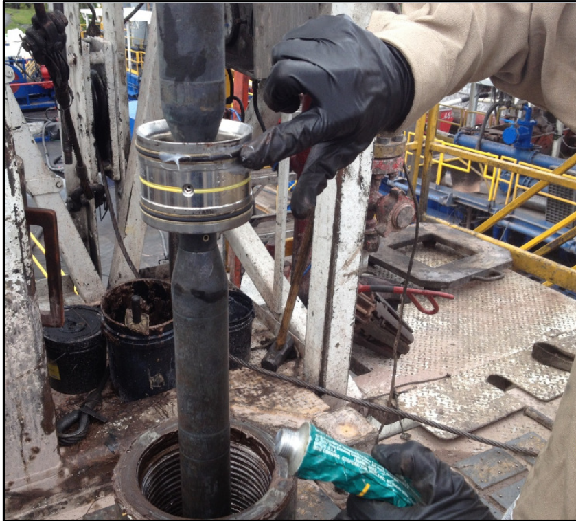
Figure 29 Grease the “O” Rings
