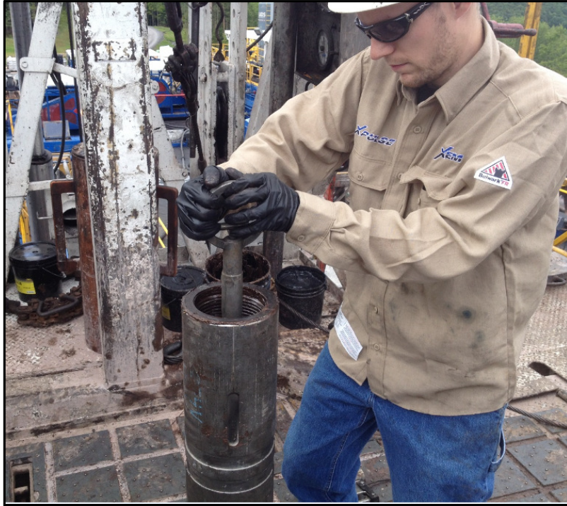
Figure 30 Align the Landing spider key slot with the Gap Sub key
