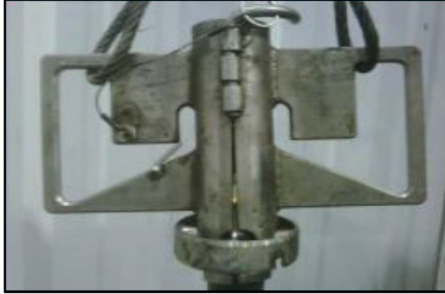
Figure 10 Legacy Pick up plate installed incorrectly
