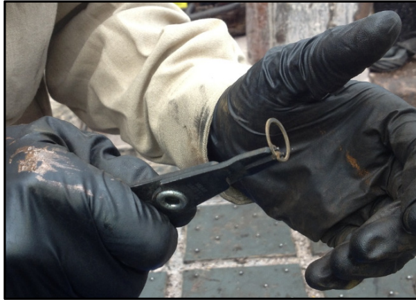
Figure 42 Snap Ring and Snap Ring Pliers
