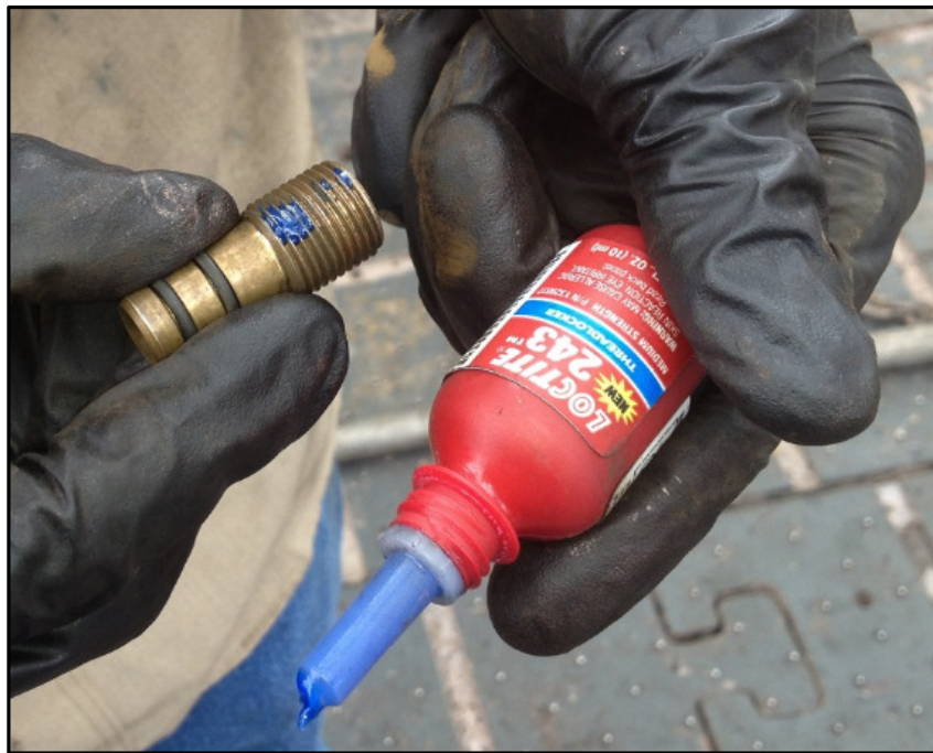
Figure 39 Smear Loctite 243 on the Setscrew
