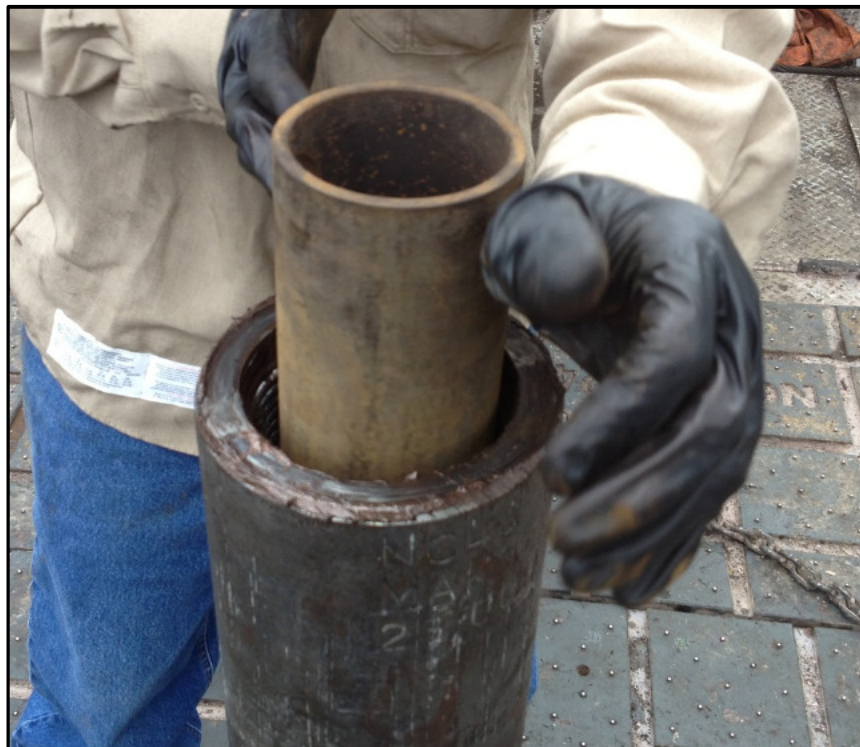
Figure 36 Castle ring Tool applied on the Castle ring
