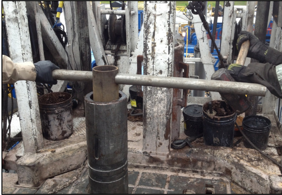
Figure 37 Torque the Castle ring
