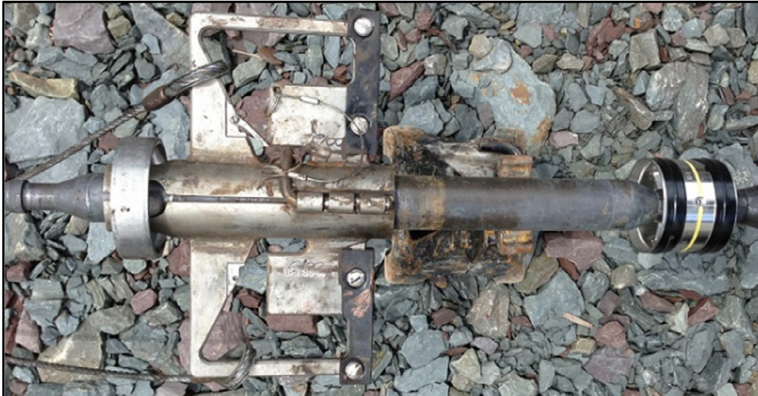
Figure 11 Pickup plate assembly installed on the DPG
