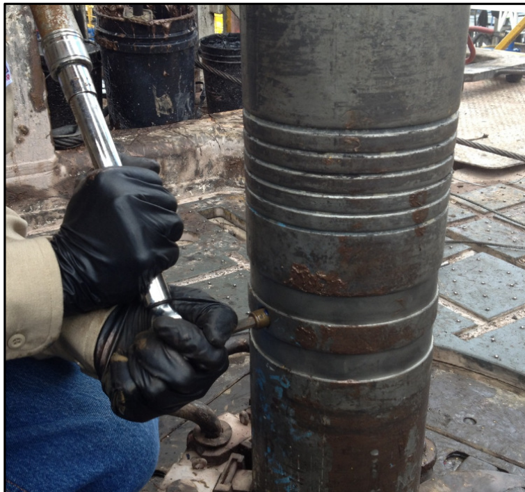
Figure 41 Torque the Set Screw
