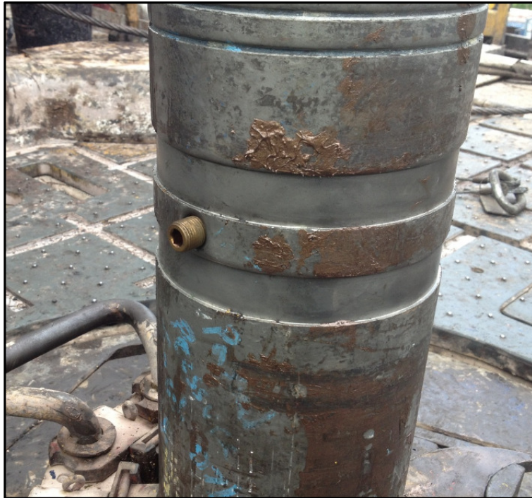
Figure 40 Grounding Set screw added to the Gap sub
