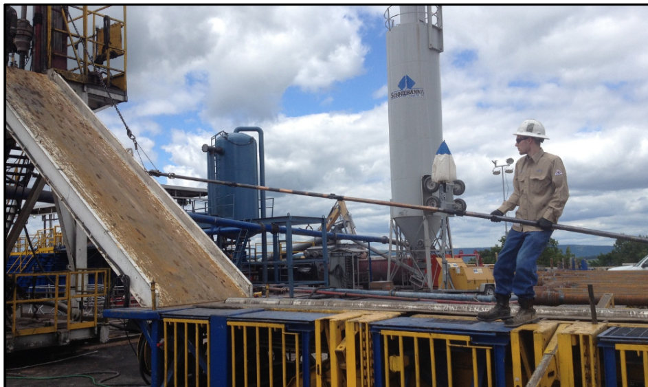
Figure 18 picking up the XEM from the Cat walk
