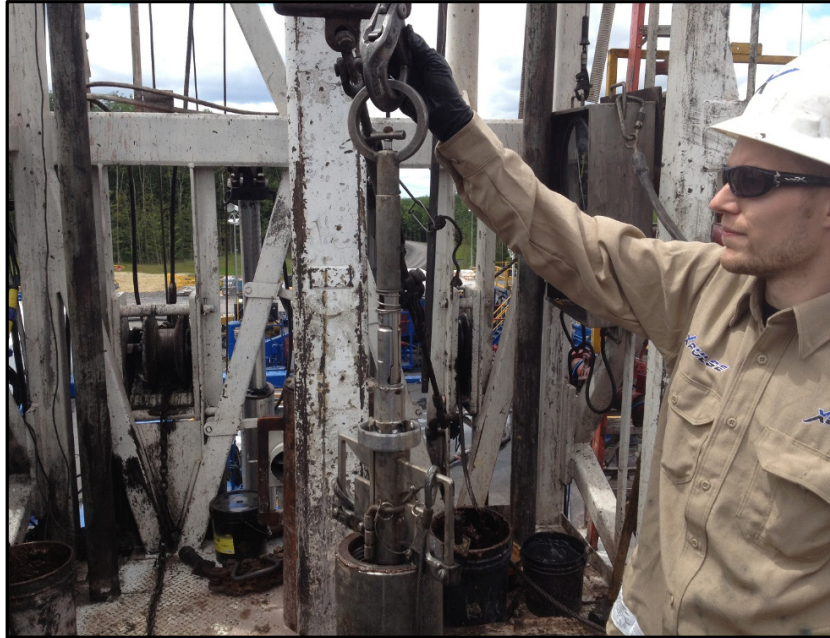
Figure 26 Overshot Attached to the DPG
