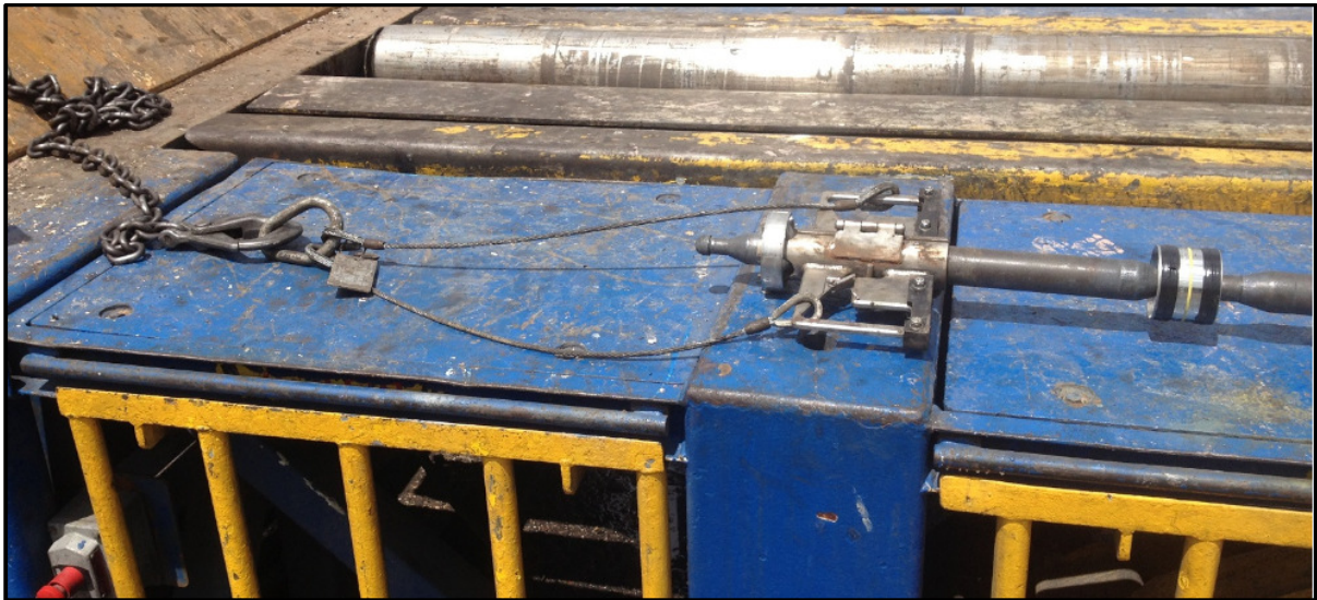
Figure 16 XEM on the Cat Walk ready to be picked up
