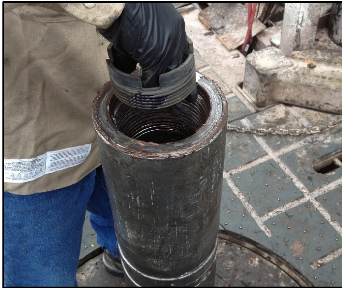
Figure 34 Castle ring installed in Gap sub
