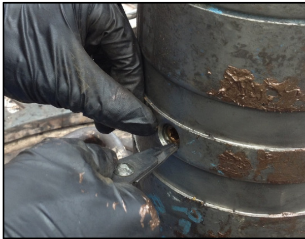
Figure 43 Snap Ring being installed
