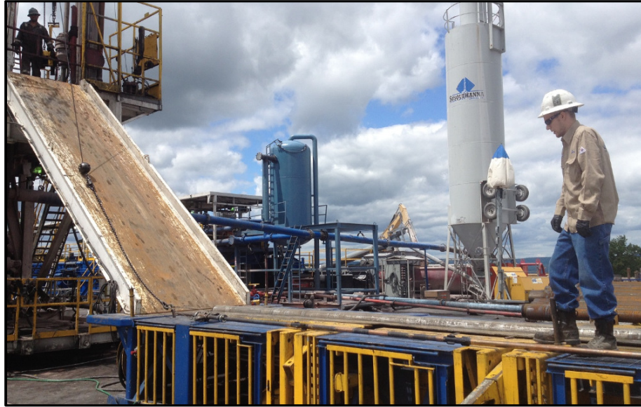
Figure 17 Pick up the XEM from the Cat walk
