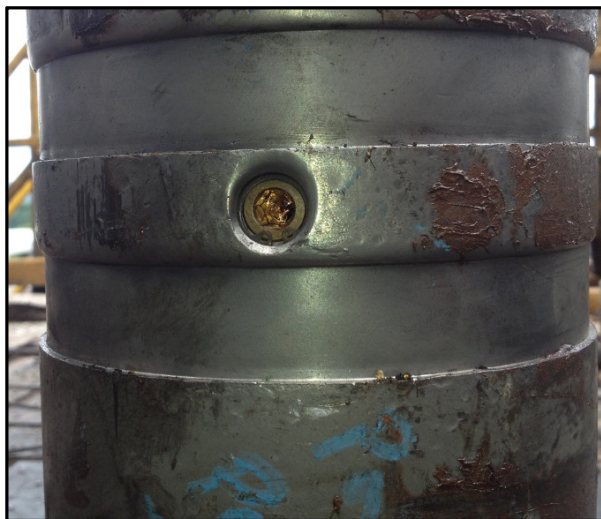
Figure 44 Snap Ring installed
