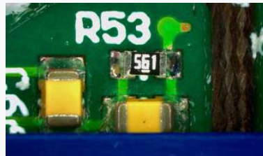
New component installed properly
