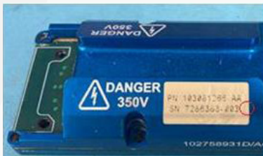
PSPD Board and cover with visual marking after modification
