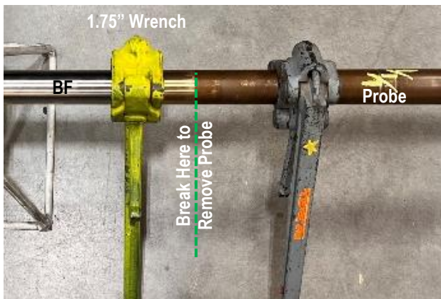
Remove attached probe from female end with centralizer removed
