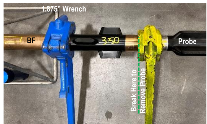
Remove attached probe from male end with centralizer installed
