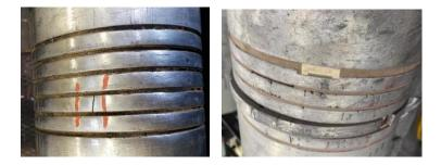
This cracking has been observed to propagate with continued use and result in pieces of the bands being left downhole. The dielectric is also then left without protection and subject to accelerated abrasion.
